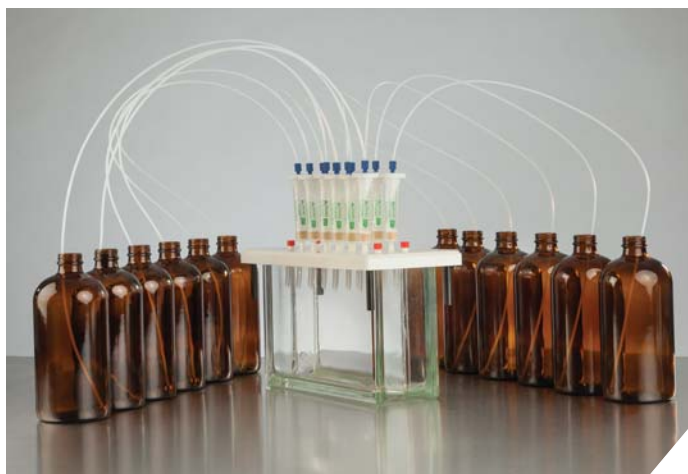
Solid Phase Extraction Setup for 12 Water Samples
